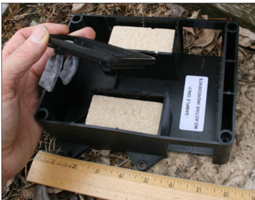
The cover of this tick box has been removed to show the inside.
