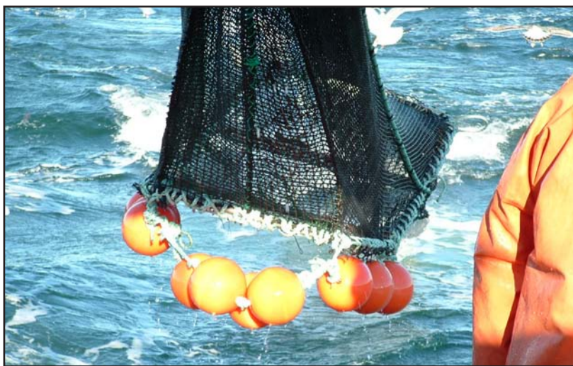
Kelo Pinkham's hinged compound shrimp grate at use aboard the Jeanne C, right. Above, floats are needed to support the weight of the stainless steel grate and to keep the escape panel open.
