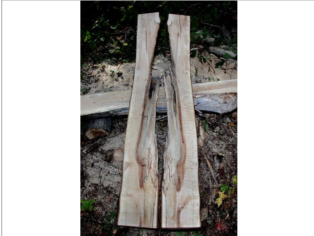
A larger split fork in ash observed 4 years after the storm with localized discoloration and decay on one face.
