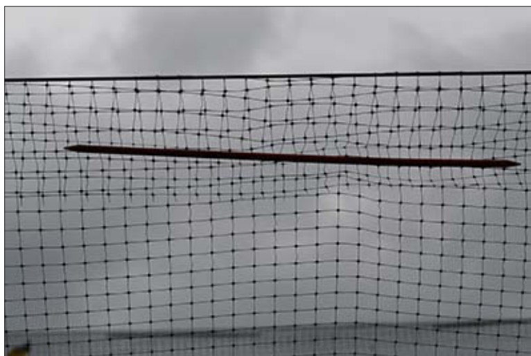
This is extruded black plastic netting, 3/4 inch mesh.
