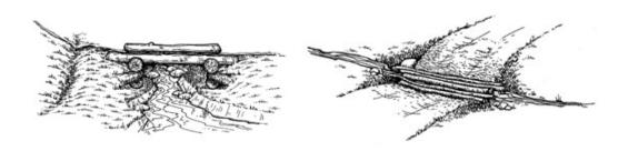
Stream-crossing structures can be temporary or permanent. Pictured here are two temporary structures. On the left, a skidder bridge and on the right a poled ford.
