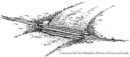
and reduced aquatic animal passage. Corduroy (poles, logs or brush laid perpendicular to the direction of travel), used to fill wet places that aren't streams, aren't considered poled fords and may be left in place.
