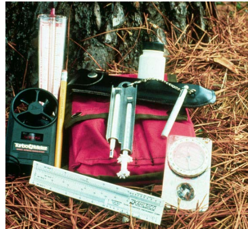
Figure 25. Basic fire weather kit: wind speed meter (two types; left center and top left), sling psychrometer to measure wet and dry bulb temperature (center), psychrometric slide rule to calculate relative humidity (bottom), and compass for wind direction (right). Photo by Dale Wade, Rx Fire Doctor, Bugwood.org.
