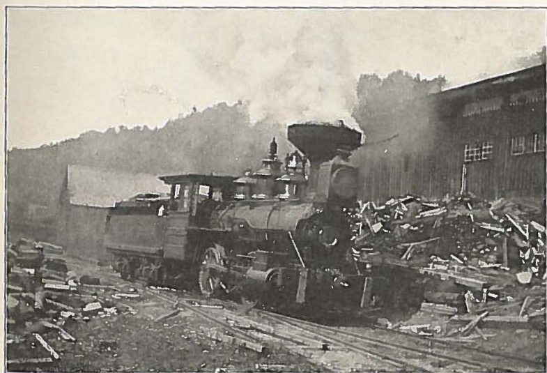
FIG. 2.—WOOD BURNING LOGGING ENGINE WITH AN EXCELLENT SPARK ARRESTER.
