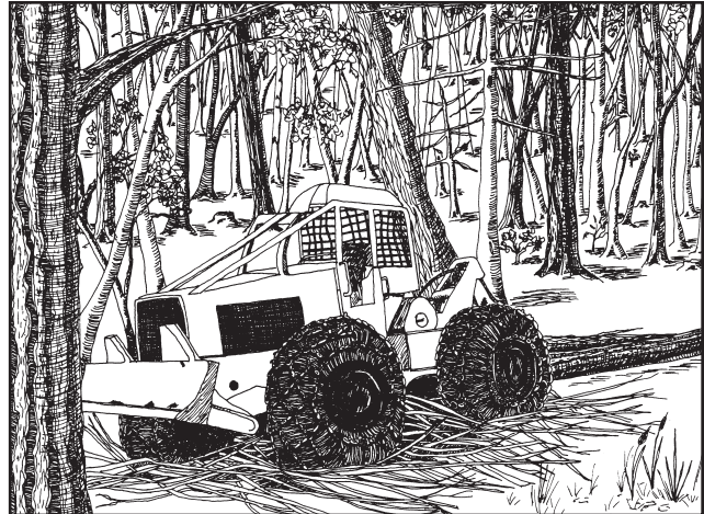
Cable skidder driving on limbs and tops.
